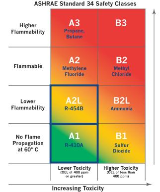
As an added precaution, Day & Night will add safety features in all systems containing R-454B which could include leak detection sensors and mitigation procedures.
